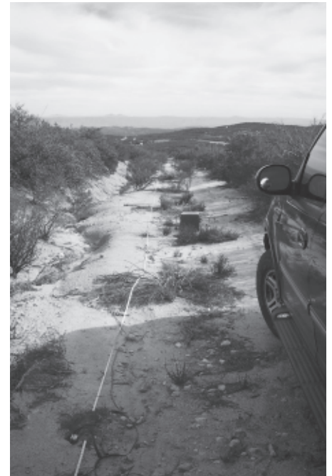
A refraction seismic line ready to read. The small object in the foreground is a geophone. The box in the center is the seismograph.
