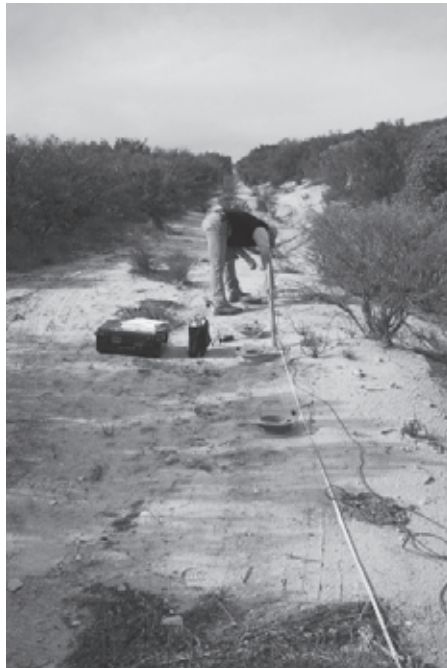
Setting up a Wenner array resistivity line. Here, the electrode spacing is about four feet.
