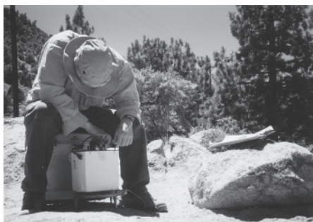
A Lacoste & Romberg gravimeter in the field.
